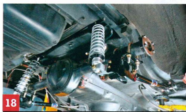
16 The connection point on the billet shock absorber mount is set 13.5 inches from the top connection point and the distance between the centre of the axle and upper wheelarch is measured. The billet mount is adjusted to match the desired ride height as determined before starting the job.
