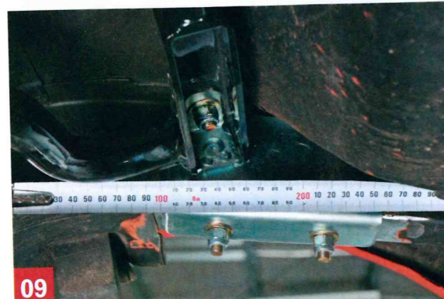
07 After the body has been stitch-welded, the cradle is bolted into place at the old position of the bump stop and at the shock absorber mounting points, as shown.
