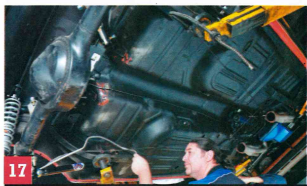
15 The housing is automatically positioned correctly when the rear ends of the upper and lower links are attached to the axle housing. Here's what it looks like with the links bolted in place. It has to remain supported until the shock absorbers are fitted.
