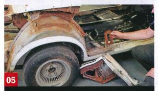
The B-pillar support has been preserved. It's sandwiched between inner and outer sill panels and serves as a guide when fitting the new panels. This is drilled because they will weld through the holes to secure the new panel. Look at the rust. And this is a clean car!
