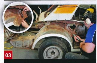
The section shown in the inset was cut away with a power hacksaw and removed so that the inside section at the pinch join between both halves of the wheel well could be reached and cut as shown.
