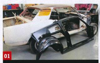
This is a Quarter Doorframe Assembly. To fit one to each side of a car, the body needs to be held in a jig otherwise it would distort due to the amount of metal required to be removed.
