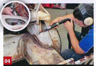
The boot hinge is next, along with the boot divider under the rear parcel shelf, as shown in the inset.
