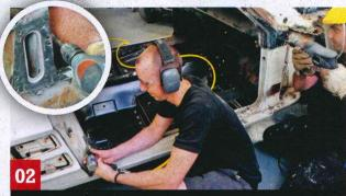
Shane (left) is drilling out spot welds in the B-pillar support. This very important area must be retained. The inset shows the opposite support from the inside. George is drilling out spot welds that attach the lower outer skin of the A-pillar to the body sandwiched in behind the upper door hinge.
