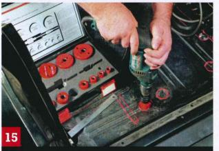
Create the new holes with a hole saw. Just get the size you need which in this case is 35mm
