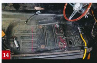
The first pink line 25mm back from the original spot weld line represents the centres of the original front access holes. The next pink line back is the position of the new weld line. Access holes will be about 25mm back from that
