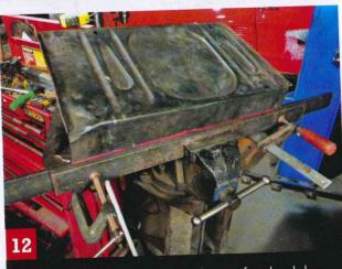
To fold, get two long, straight heavy pieces of steel and clamp them in a decent vice like this. You can use heavy angle iron or flat bar with flanges welded on to keep them level with each other in the vice jaws as shown here
