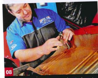
The seat box is re-attached to the seat to determine the exact position into which it will have to be welded
