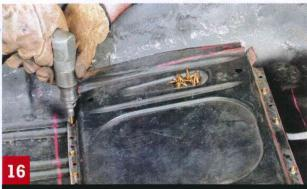
Drill holes along the new flanges about 37mm apart. Then fit Tek screws through the flanges between the holes you drilled to firmly clamp the seat box to the floor pan, tunnel and sill
