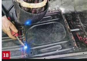
Make 'puddle' welds through the drilled holes onto the floor pan, tunnel and sills
