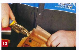
The curved side of the transmission tunnel will prevent the seat box from dropping into the lower position. The corners between the flanges will need some detail bending that can't be done in the straight edges
