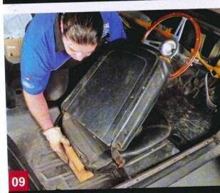
Because there are no spot welds holding the seat box in place, the rear of the seat must be supported
