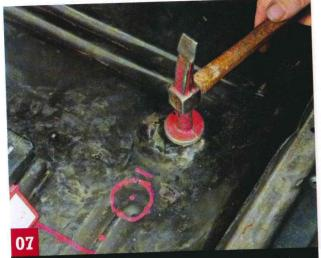
Discs are tack welded until the edges are completely sealed. Use a panel hammer to flatten the area across the plug
