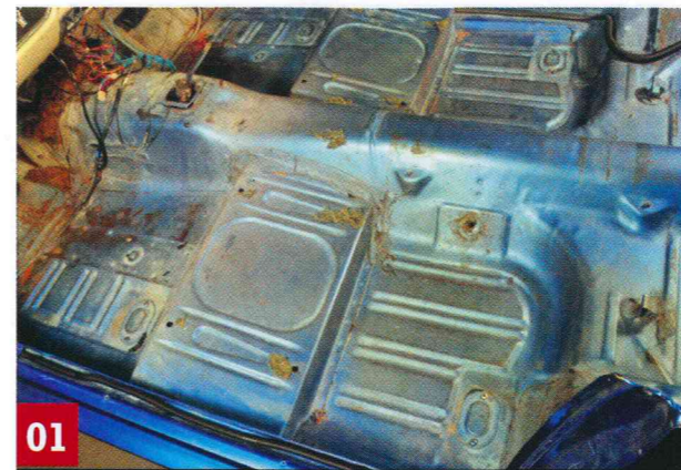
01 Standard interior of a stripped-out Mustang. The seat boxes have to be removed, altered, and refitted in a better position
