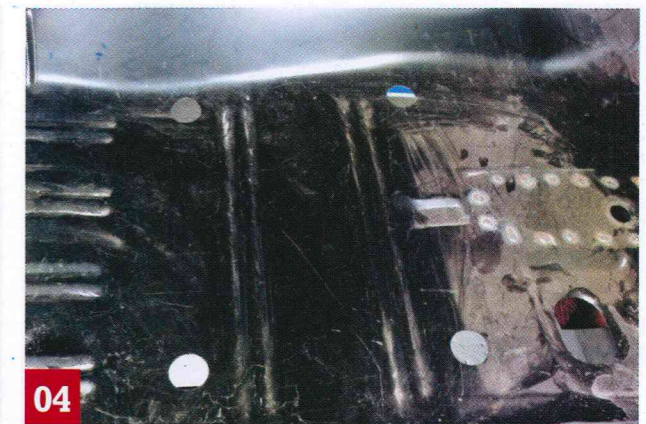
04 Four holes in the floor that allow access to the seat retaining nuts. When the seat boxes are removed you'll see them
