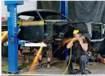
To remove the floor, use the tools you prefer; cutting discs, power hacksaw, even oxy or plasma-cutters for the heavier sections. Given the scope of material removal, it's essential the car is completely stripped of anything flammable, such as fuel lines and carpets. MCF removed the sections in manageable chunks as having the whole lower half of the car fall away as one would be quite dangerous.
