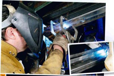
Despite bracing, the sills still tend to bow outwards near the centre. These bowed sections need to be pulled (clamped) in tight against the chassis before welding. Weld each side alternately and start in the middle, progressively working towards the ends. The Challenger's inner sill is canted, creating a gap at the top. A steel strip was shaped to follow the factory pressing, then welded in place to bridge the gap.
