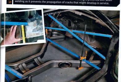
Ideally you want the rails to sit nearly flush with the bottom of the sill panel. MCF positioned the cross bracing so that it held the body at the desired height. Using specifications supplied when ordering the chassis, final ride height is determined by the amount of kick-up in the front and rear of the chassis — this is preferable to sinking the body down over the rails. Adjustable shocks can fine-tune the stance.
