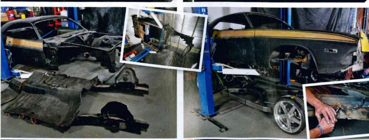
The chassis are manufactured to precise tolerances and fit very neatly between the inner sills. Therefore any material that isn't removed will prevent an accurate fit and could cause misalignment of the body. It's impossible to get it all in one go, no matter how good you are, so you'll have to go back and clean up a few areas before you're able to get the body sitting snuggly over the new rails.
