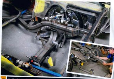
Unlike the bolt-in nature of the GT Sport, Morrison supplies the Max G with generic front and rear sections due to the variations in fitment and design. This means parts such as radiator support panels, fender mounts, fuel tanks and bumper bar mounts will require some finessing and fabrication work. Here, the MCF team had to kick the front rails out around the front wheels to align with the factory mounts.
