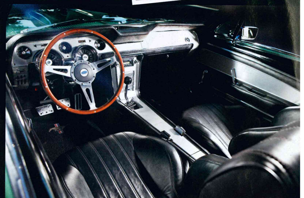
INTERIOR: The TKO's adjustable shifter location means it can be positioned perfectly so that it emerges out of the factory console smack in the right spot
