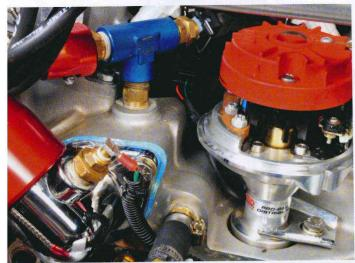
The MSD dizzy and 6AL box were retained but modified — the advance weights and springs were removed and the advance plate locked at zero; the ECU now controls advance and retard. A Hall effect sensor was added inside the dizzy so the ECU can calculate the internal position of the engine, allowing it to fire the appropriate injectors at the correct time, which in this application is in pairs across the engine.
