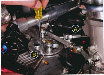
Trim the outer cable (sheath) to length and slip it into the adjustable collar (A). Then feed the inner cable in, guiding it around the slot and through the small hole in the barrel-shaped clamping pin (B). Use pliers to slightly tension the cable, then tighten the clamping pin. Fully depress the accelerator pedal and check the throttle plates are wide open. If they're not, the accelerator pedal angle will need adjusting inside.
