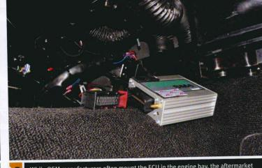
While OEM manufacturers often mount the ECU in the engine bay, the aftermarket has found the interior's cooler and drier environment to be preferable. Here, the Autronic SM4 was mounted to an out-of-the-way bracket beneath the front of the console. It's completely out of sight when the console is refitted, yet remains quite serviceable. Be sure to use a grommet when running the loom through the firewall.
