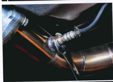
An oxygen sensor isn't strictly necessary but it's a good idea to fit one for each bank of cylinders. Apart from the usual advantages, their fitment allows Autronic's 'auto tune' to be activated. Once configured, this can be used to get a pretty decent map up and running. It's no substitute for a comprehensive dyno tune but it will get you to the dyno. Note the coolant temp sensor at the back of the blue T-piece in Step 13.
