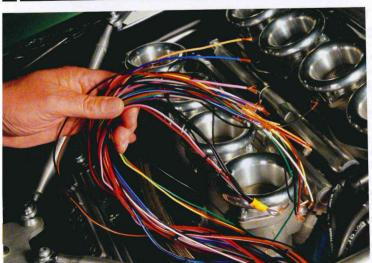
The wiring diagram supplied by Autronic matches the colour coding of the wires, and the connections are fairly straightforward. The abundance of wires reflects the wide variety of things the unit can do — many functions will not be used, so many wires will remain unconnected. Basic connections are injectors, ignition, power, earth and fuel pumps, plus throttle position, coolant temperature, MAP and oxygen sensors.
