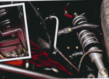
A 3/8in line is the minimum for performance applications. Mick's tough Mustang already sported an upgraded supply line but needed a return line. When routing lines, keep them near underbody areas that provide shielding and use cushioned P-clamps to keep them secure and clear of moving components. Sections of hardline joined by rubber hose should be flared and clamped on either side.
