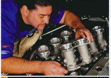
It is possible to assemble the throttlebodies and the fuel rails onto the manifold prior to installation. However, for this installation it was simpler to bolt them up once the manifold was in place. Here Leo (proprietor of the Muscle Car Factory) is dropping the throttlebodies in place. Be careful not to over-tighten the mounting nuts or you risk distorting the bases of the cast alloy throttlebodies.
