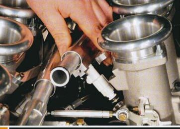
Each injector rail is supplied in two halves that slip together — they seal via the visible O-ring. Installation is easiest if you attach the injectors to the rails and set them in place as you attach each pair of throttlebodies. Injectors are supplied with the kit; when ordering, give TWM your engine and cam details so they can calculate your basic fuel requirements and supply suitably rated (flow rate) injectors.
