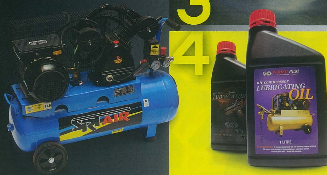
4 FAR LEFT: You can never have too much air. Compressors should only run at 50 per cent duty cycle. If too small they'll run constantly and wear out. About 320l/m (11cfm) is the biggest you can plug into 240V. A bigger tank helps
