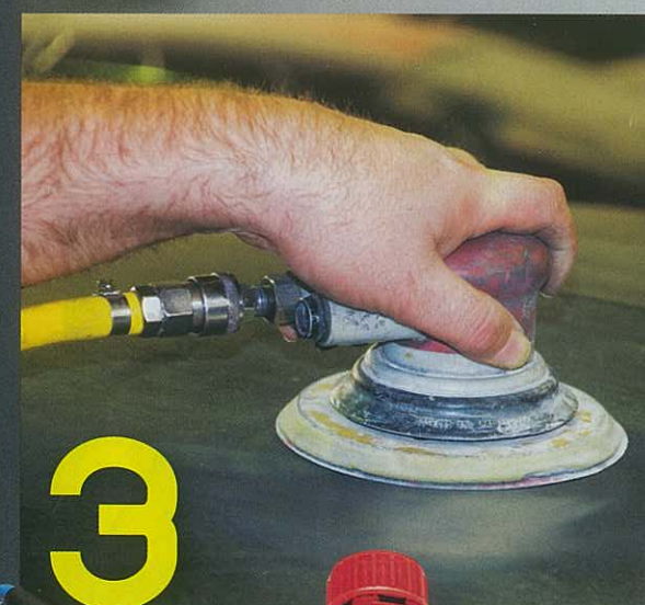
3 Dual-action air sanders are standard issue in any body shop though they're only suited to near-flat panels and won't get into tight corners. They make a lot of dust and consume lots of air
