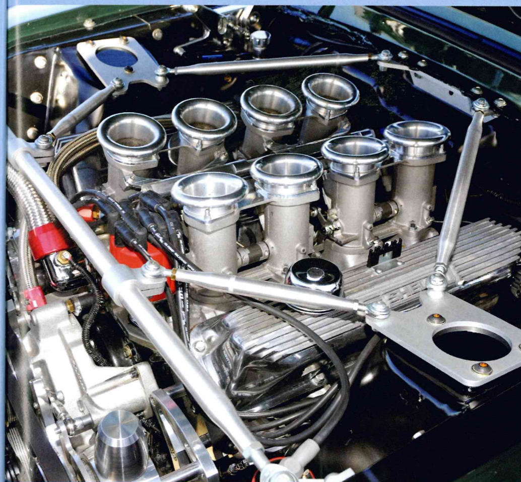
Above: What a surprise you get when lifting the bonnet of Michael's cool Fastback. That injection speaks for itself and sits on top of a well-detailed, 540-horsepower 427ci "Side Oiler" big block.
